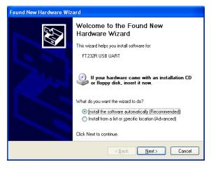
If this is the first time you have attached the USB interface to your computer, the "Found New Hardware Wizard" will start up. For now select "install software automatically".
